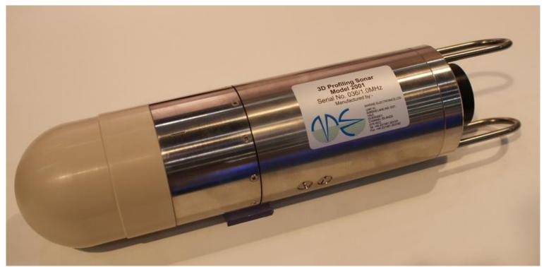
The 3D Profiling Sonar Model 2001-90 is designed to operate long term in enclosed spaces including radioactive ponds and settlement tanks and gather high resolution bathymetry data. Manufactured in PEEK / Stainless Steel and only 90mm in diameter the unit can be installed through the smallest of access points. Multiple units can be linked together and controlled via Ethernet to enable large areas to be fully mapped. The windows software allows images to be merged to produce a single point cloud
